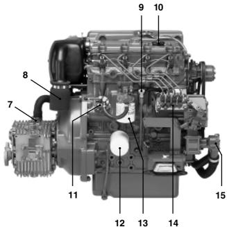
D2-55 with reverse gear MS25L
